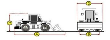
C. Height (ft and inches) 12'6" D. Shipping Width (ft and inches) 11' 1/2" Operational Weight (Ibs)
