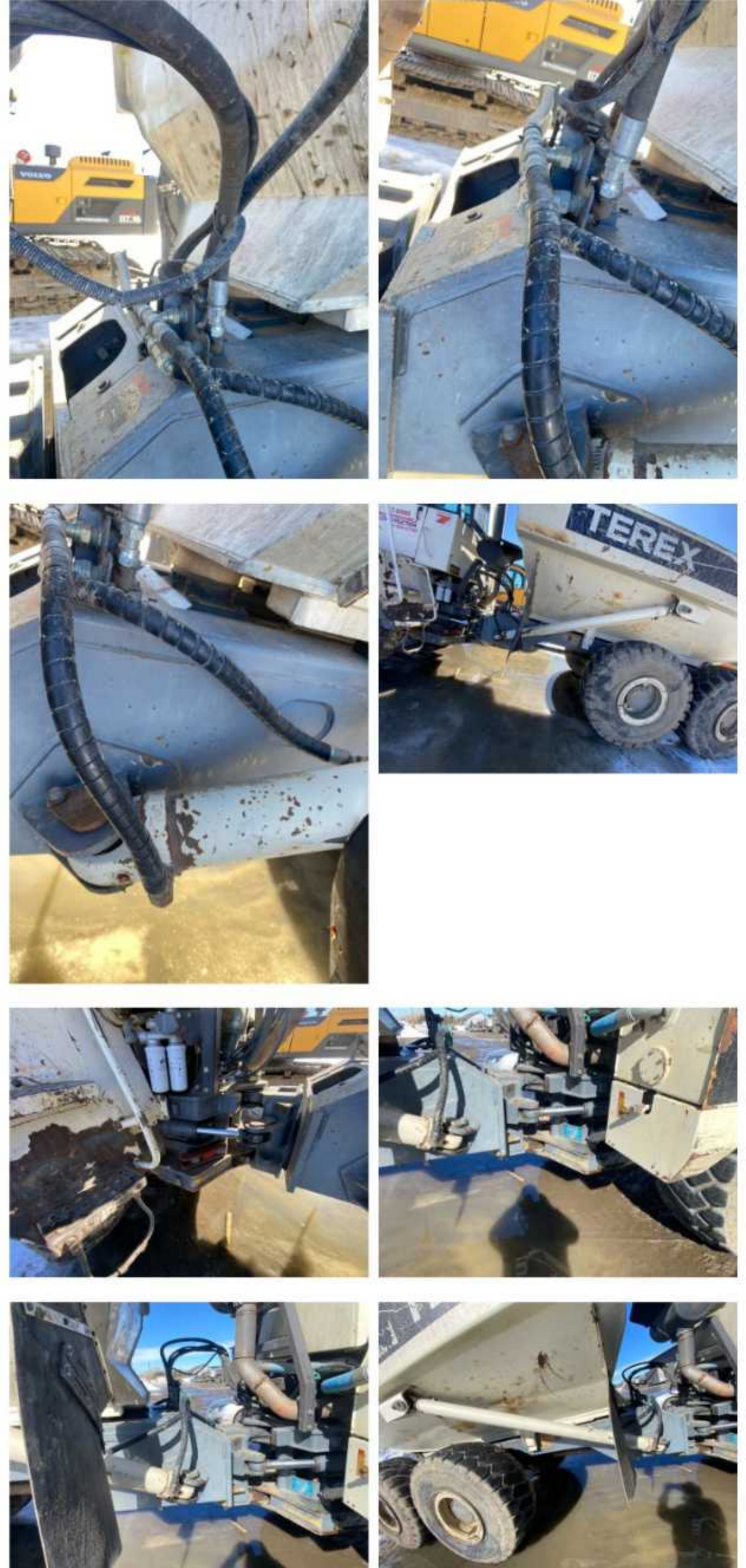
Hydraulic Leaks Photos
